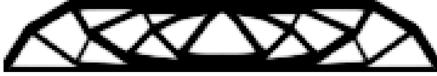
Figure 5.3: A reference optimal topology for the MBB beam discretized using 180 \times 30 elements.
