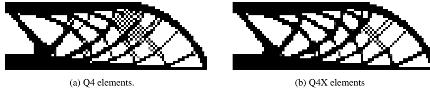
Figure 7.5: Optimal topologies of the MBB beam using symmetry and employing (a) Q4 and (b) Q4X elements.
